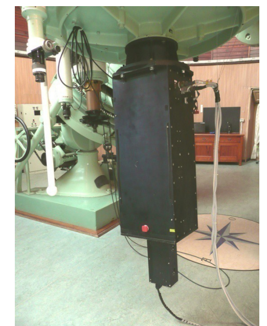
PISCO at the Cassegrain focus of the Zeiss telescope of INAF-OAB at Merate
